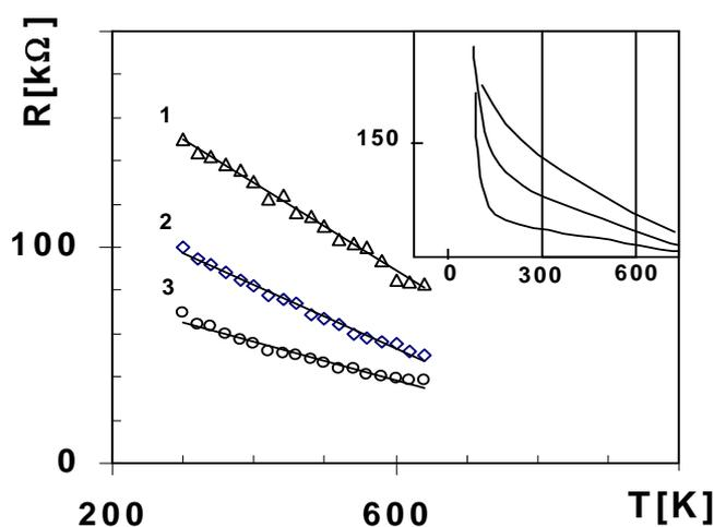
Fig. 4 The linear segments (300-600K) in the temperature dependence of resistance of samples. The insets depict the general exponential behaviours of resistance. For these compounds, the resistance jumped over  $10^3 \text{k}\Omega$  in lower temperature range.
