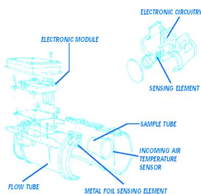
**Fig.2** A block-scheme of a hot-film MAF sensor
