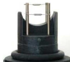
**Fig.1** The arrangement of the Pt wire in the Hitachi hot-wire MAF sensor (real size)
