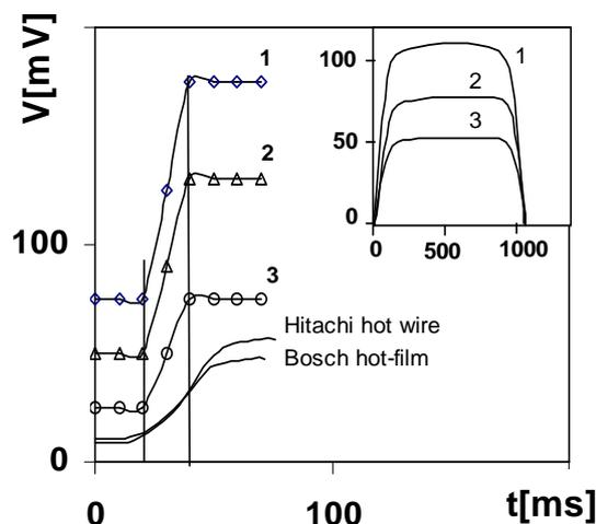
Fig. 7. The time response in the 1m/s velocity change. The insets show the system reaction to a sudden 1s start-stop of a 1m/s flow
