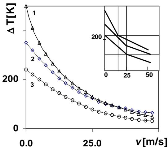
Fig. 6 The exponential decay of the temperature gradients on the air flow velocity. The insets show the linear response approximation segments. The input current needs to be adjusted to keep these segments within the desired temperature range
