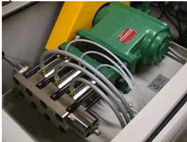
Figure 4: Crankshaft pump (Courtesy of OMAX Corp. Kent, WA)
