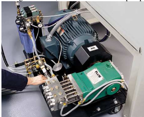
Figure 2: Direct pump (Courtesy of Flow International Cooperation)
